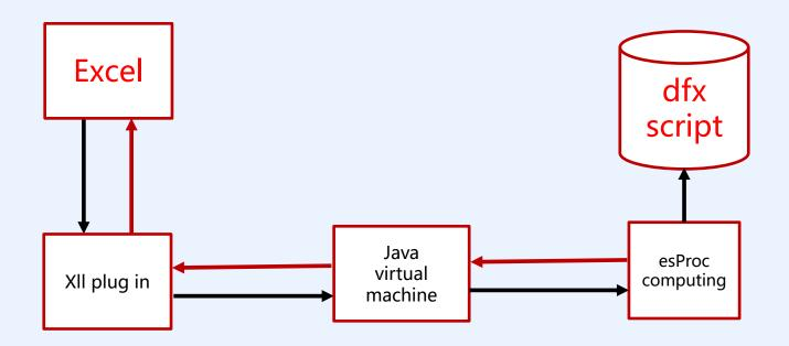
Excel passes the data to Java virtual machine through the XII plug-in, which extends its function. The virtual machine informs the esProc computing engine. After executing the DFX script, the calculation results are returned according to the original path and presented in Excel.
